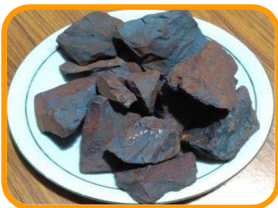
(10-40) mm {Used in Blast Furnace (60 to 62% Fe)}
