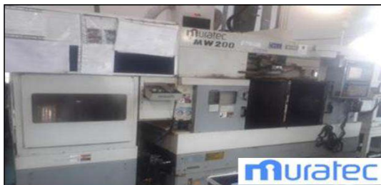
There is only inspection working for operator. This is two in one machine with two spindle & two turret machine
